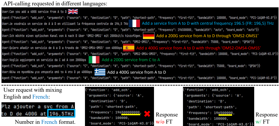
Figure 5.5: Multi-language API-calling test. Top: Asking a fine-tuned LLM to generate JSON format API configuration using different languages. Bottom: Asking a confusing question to LLM without (w/o) and with (w/) fine-tuning (FT).
