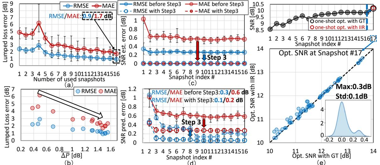
Fig. 4. (a) Lumped loss estimation accuracy; (b) Correlation between lumped loss estimation accuracy and power variation; (c) SNR estimation without/with step 3; (d) SNR prediction without/with step 3; (e) Optimized network margin (top) and optimized SNR of all services (bottom).
