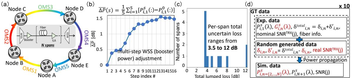
Fig. 3. (a) 5-OMS ring network; (b) Average booster power variation; (c) Histogram of total lumped losses; (d) Data usage assumption.
