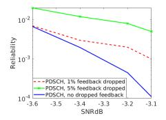
FIGURE 12. SPS PDSCH transmission's reliability in latency of 1ms with dropped feedback and no dropped feedback.
