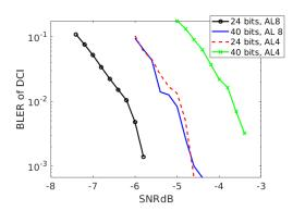
FIGURE 4. Block error rate of Release 15 DCI with 40 bits payload and Release 16 DCI with 24 bits payload.
