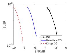
**FIGURE 3.** Comparison of UL transmission performance in DG transmission, reactive CG transmission and K-repetition CG transmission.
