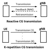
FIGURE 2. UL repetition CG transmission.
