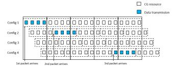
FIGURE 10. Multiple configurations to ensure K repetitions.
