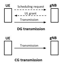
FIGURE 1. UL DG and CG transmission.
