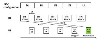
FIGURE 11. DL SPS transmission's HARQ feedback cancellation DL SPS transmission in TDD.
