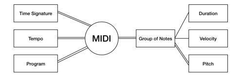
Figure 11.1 – Schema of the graph generated from MIDI. The double lines represent links of type many-to-many.
