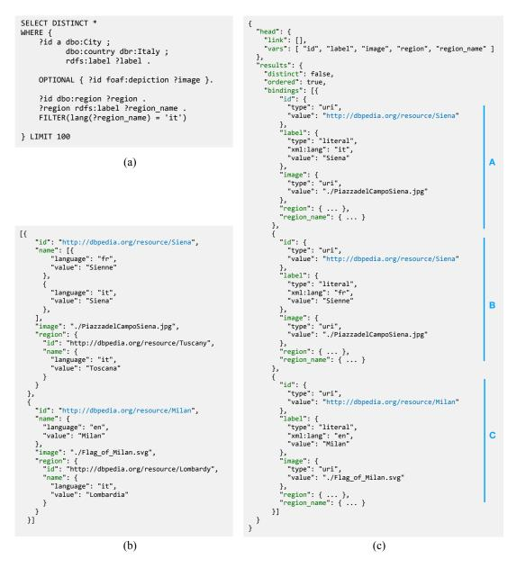
Figure 6.1 – A SPARQL query (a) extracting a list of Italian cities with picture, label and belonging region, of which the URI and the Italian name are also requested. In the standard output of the endpoint (c), the city of Siena is represented by both object A and B, while the transformed output (b) offers a more compact structure.
