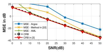
Fig. 2. Comparison of single antenna transmit schemes with the CRB (G = M = 16).
