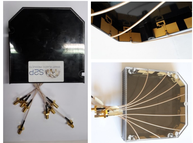
Fig. 1. Pictures of the LDS antenna prototype
