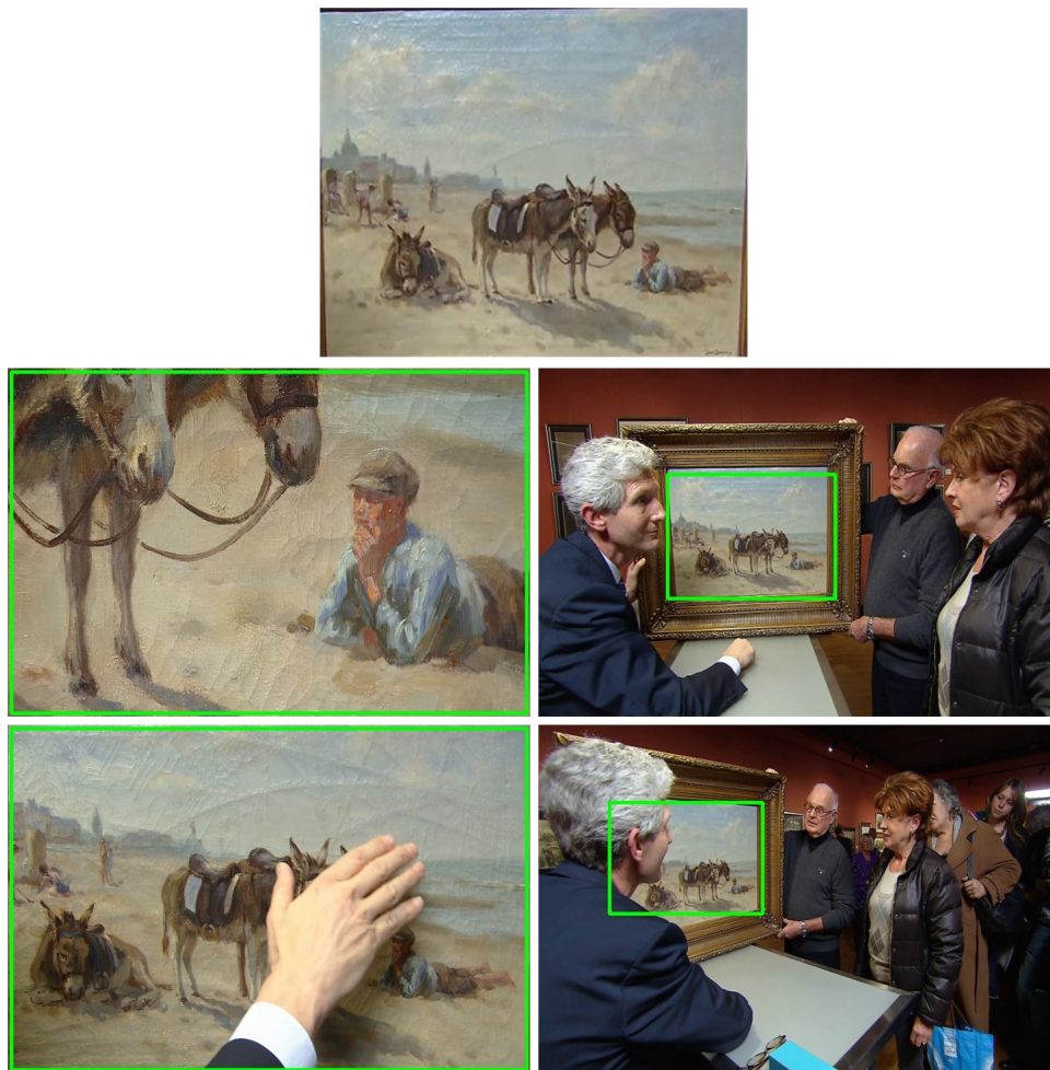
Figure 3.5: Object of interest (top row) and in green bounding boxes the detected appearances of it, after zoom in/out (middle row) and occlusion-rotation (bottom row).
