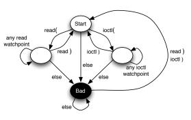
Fig. 5. A portion of Sherlock's Büchi automaton used to distinguish between benign and suspicious operations. All states are accepting. The figure shows the portions of the automaton corresponding to the system calls read and ioctl; the patterns for other system calls are similar. Whenever the automaton enters the *Bad* state, the internal kernel operations are not matched with a requesting system call, an indicator that an Illusion attack is underway.
