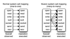
Fig. 3. System calls and examples of system call-to-operation mappings.
