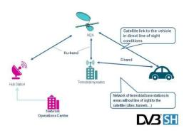
Figure 1. DVB-SH broadcast network architecture
