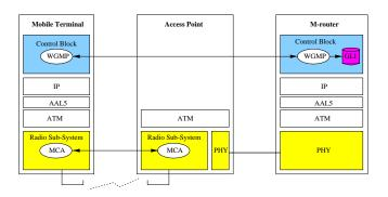
Figure 5: Architecture of WAND reference IP system.
