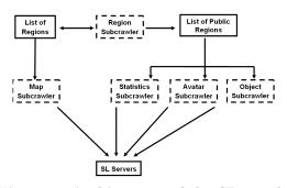
Figure 1: Architecture of the SL crawler
