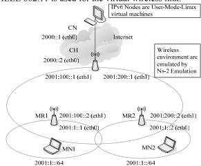
Figure 6. Virtual Wireless Mesh Testbed
