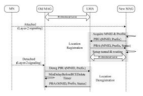
Figure 2. PMIPv6 Sequence Diagram
