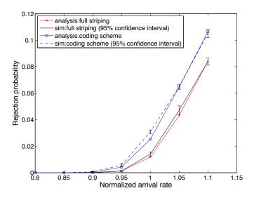
Fig. 1. Rejection probability with M=128, Video encoding rate  $R_{enc}=2Mbps$ , Upstream bandwidth  $B_{up}=1Mbps$ , Size of Video L=2Gbytes, Coding overhead  $\epsilon=0.05$ , and Maximum number of simultaneous incoming connection y=31.
