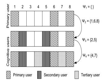
Fig. 2. One primary user and two cognitive users in a system with 8 subbands.
