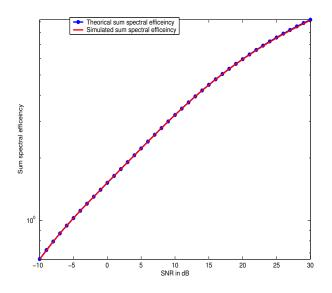
Fig. 3. Comparison between the theoretical expression of the sum spectral efficiency in (24) and the simulated one in (12) for L = 5 and N=32.
