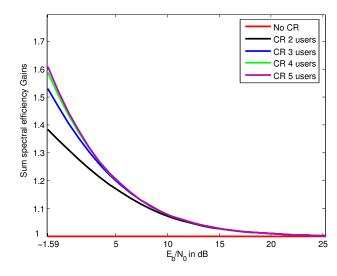
Fig. 5. Sum spectral efficiency gains of the system with 5 users.
