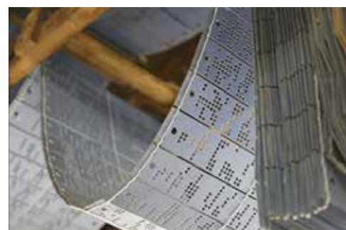
Punchcard used as a guide for silk weaving with a loom
