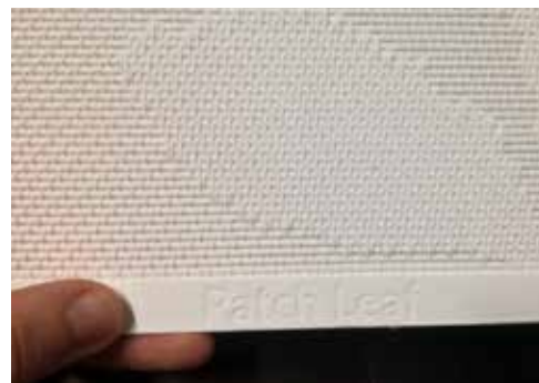
3D printing of a Damask. The example shows a leaf extracted from an image of a historical textile. As it is a damask, weft and warp yarns are of the same colour
